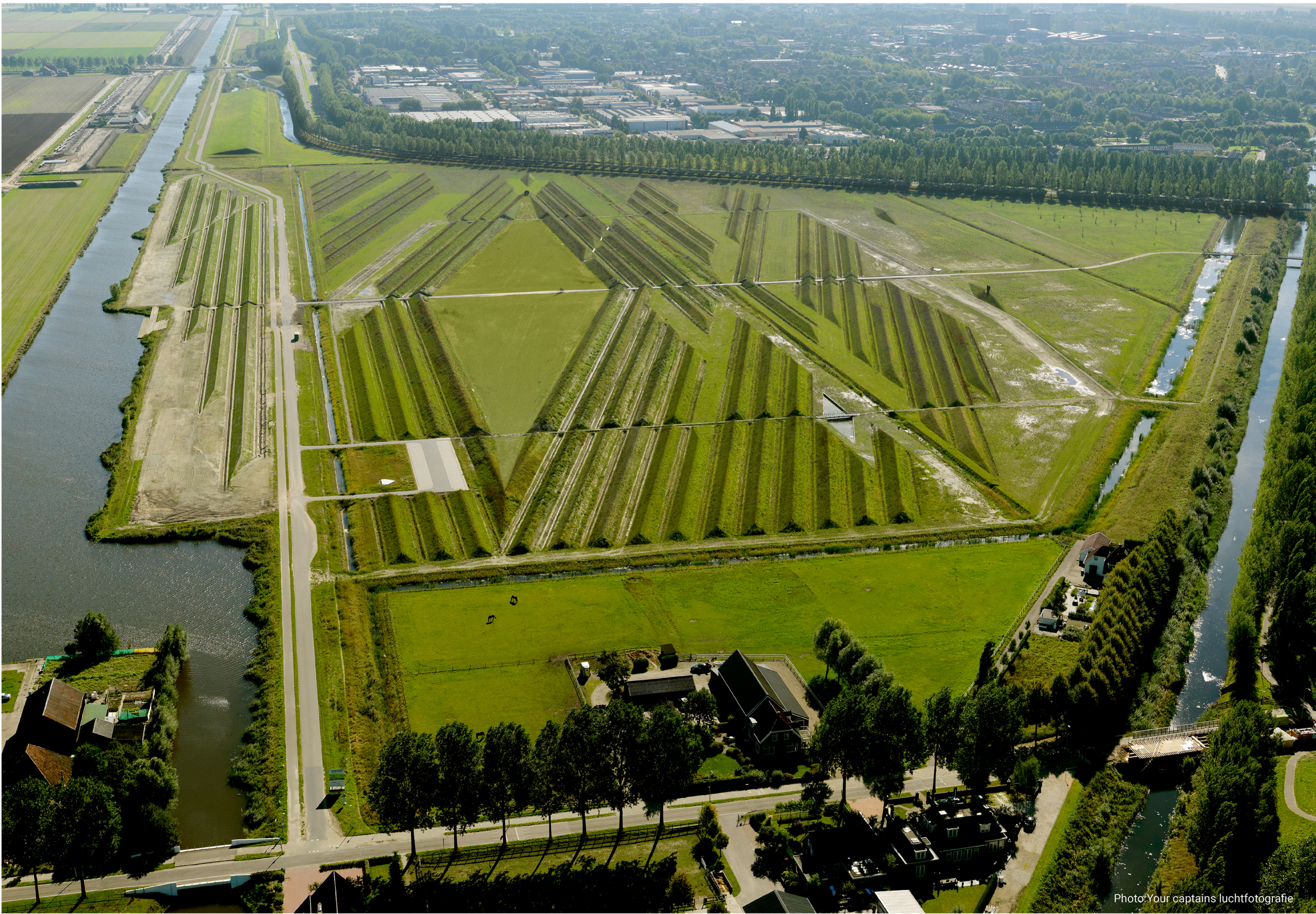
Section of the sound reducing ridges with ditches and maintenance paths, also for walking
