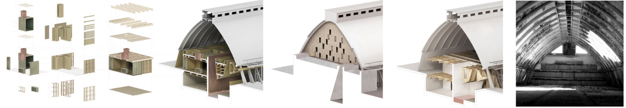
Nervi's salt warehouse: exploded views and section of the structure, the facade and a current internal view.
